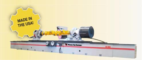
The CGX 460-4100 is suitable for rebuilding crankshafts or low productivity manufacturing.
