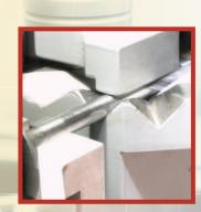
V-Ways and clamping system for accurate valve stem butt-end grinding and chamfering.
