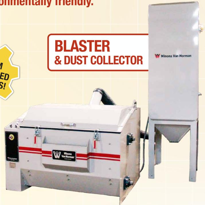
Next, the **shot blaster** uses a full-length, single-impeller motor to ensure the most consistent cleaning to bare metal and eliminating the extra manual labor.
