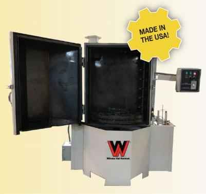
**Designed to remove oil,** grease, grime, dirt, and other contaminants off a various amount of parts.
