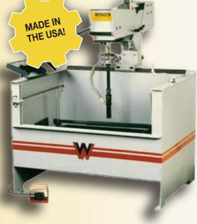
The PS3301 Power Stroke Hone is a true power stroke hone for auto and truck engine blocks.
