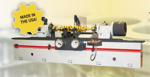
The CGX 300-2200 is suitable for rebuilding crankshafts or low productivity manufacturing.
